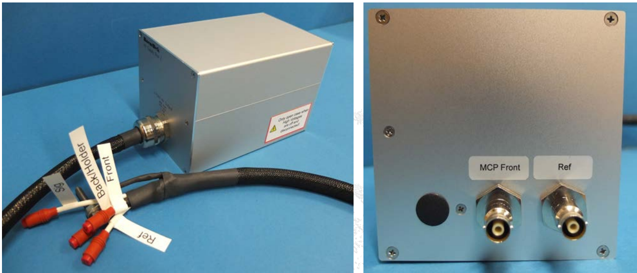
Figure 5.21: Left picture: HVZ10 box with four-fold high voltage output cable which will be connected to an XHV feedthrough. Right picture: high voltage inputs on rear panel. Here, two SHV10 socket are provided for supplying two independent voltages. Other versions are available which operate with just one input voltage (MCP front or U_{ref} ) and/or use other input socket standards
