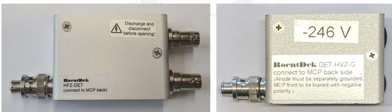
Figure 5.18 HVZ-G plug, here the version for negative bias of MCP back potential.
