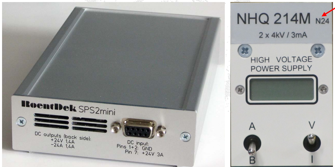
Figure 5.9: SPS2mini mains adapter (left) and the specific label (red arrow) on the front side of a “N24”- type HV2/4 module which can be powered by it (those units with side panel labels will show the N24 indication there). The N24-type HV modules can also be operated with old-type NIM-crates that does not supply the \pm 6 V.
