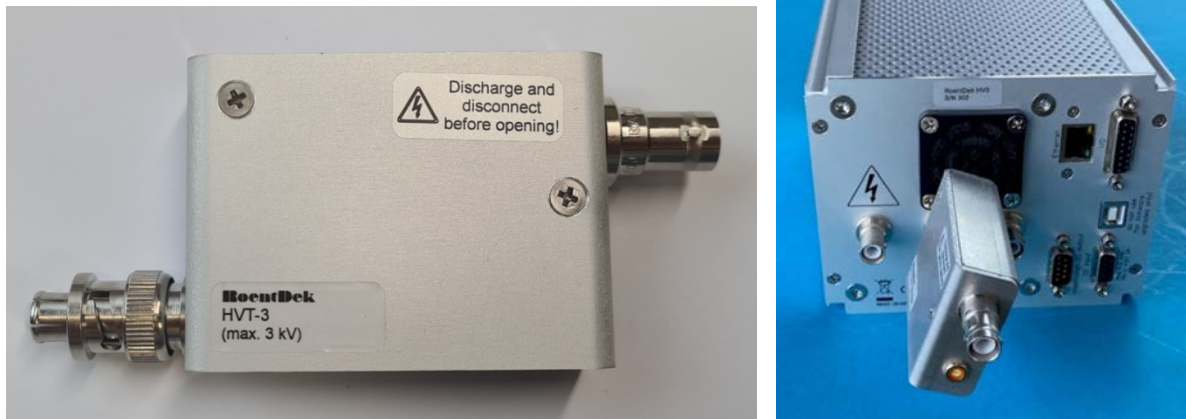
Figure 5.13: The HVT-3 can be directly connected to the output socket of a high voltage supply.
